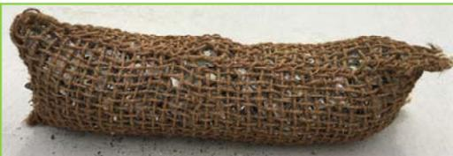
An 'Oyster Reef Sausage' made of biodegradable coconut mesh and filled with waste oyster shells from commercial leases. Baby oysters will grow amongst the shells and glue them together, before the coconut mesh degrades away, revealing a newly formed oyster reef within the Noosa River! Each new oyster reef will be made of nine of these 'sausages'.
